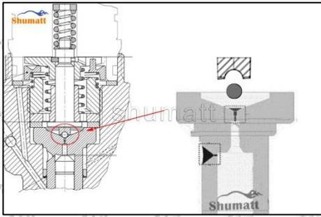
(3) (3) When installing the valve stem, make sure that the valve stem and the bonnet must ensure that the valve stem can move smoothly in it. as below
