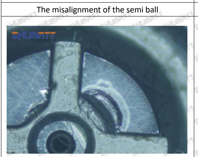
The indentation of the misalignment of the semi ball
